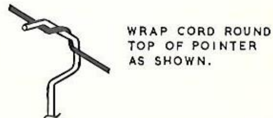
CORD DRIVE ARRANGEMENT DIAGRAM- MURPHY TRANSISTOR PORTABLE MODEL P71
